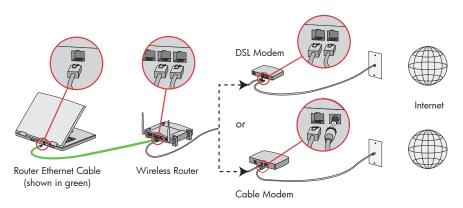
Network connections with router Ethernet cable temporarily connected (jack locations vary)
